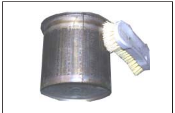
Cleaning the burner
